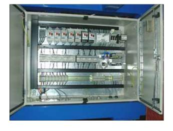
The second electrical cabinet contains all of the 415 volt three phase components, such as contactors and overloads for each of the Speedband's motors. This cabinet is also lockable ensuring maximum safety, while keeping the internal electronics safe.
