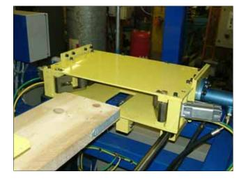
The scaffold boards are passed to this station where the hydraulic rams press the band into the sides of the board. After leaving this station the boards are stacked by the auto stacking part of the Speedband machine...
