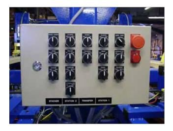
Whilst the Speedband is a fully automatic piece of machinery manual control of any function is accessible via the manual control switch box.
